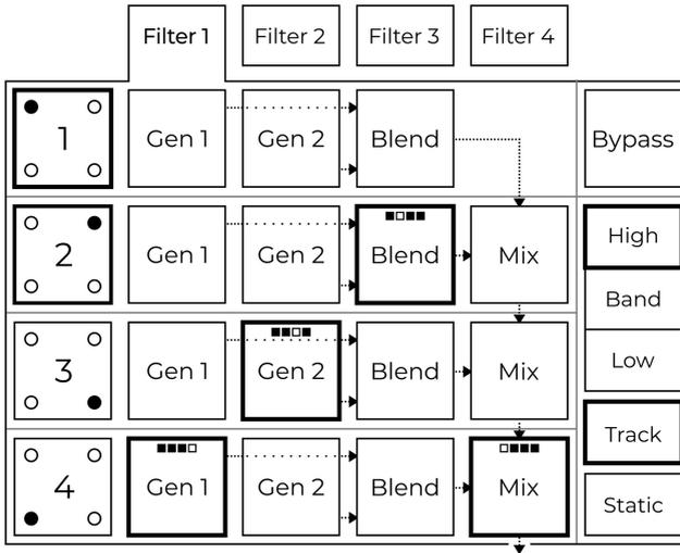
The picture above shows the Corner Matrix interface with four tabs representing each filter and four rows corresponding to each Corner.
