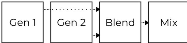
Each Corner is controlled by five parameters (**Overtone Gen 1 and 2, Overtone Blend, Filter Cutoff** and **Filter Resonance**) which are assigned to the five knobs just below the display. These knobs increase or decrease values of the selected Corners' parameters.
