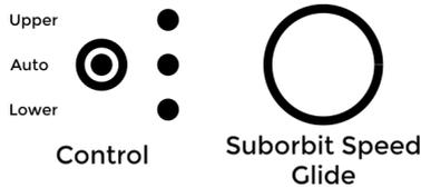
In the case illustrated above, the **Control** switch is in the **Auto** mode which means the encoder either functions as **Suborbit Speed** or **Glide**, depending on the active screen.
