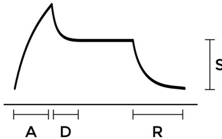
The envelope is triggered on a per-voice basis when a note is played. It is possible to choose either exponential (**Exp**) or linear (**Lin**) curve for each envelope.
