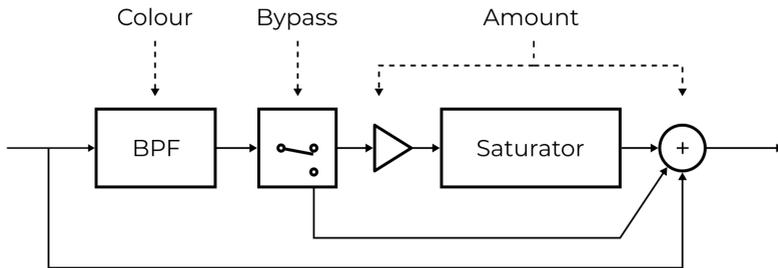
The **Bypass** button on the **Effects screen** disables the saturator. In this case, the **Drive Amount** only sets the mix level of the effect's band-pass filter.
